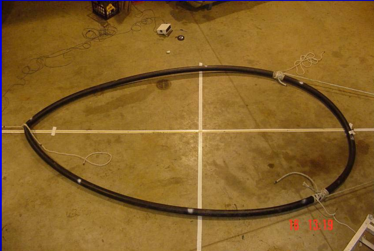
Deformed rim under load
