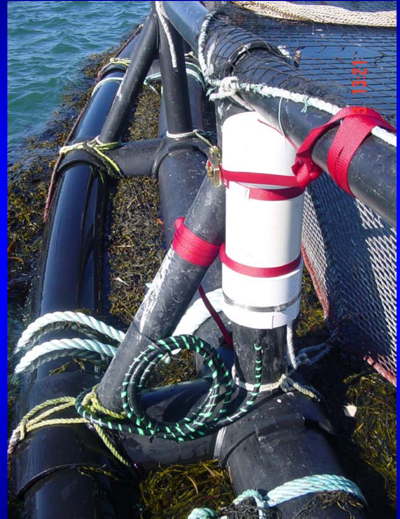
Cage Rim with attached Load Cell Data Recorder
